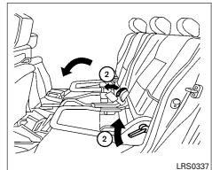
Then lift up on the recline lever on the side of the outboard seats to fold the outboard seatbacks flat. To fold the center seatback flat, pull up on the strap on the edge of the center seat cushion and fold the seatback toward the front of the vehicle.
